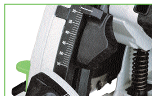
Precise and advanced: depth indicator.
