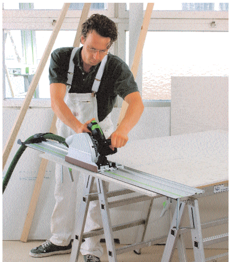
Using the TS 55 to saw MDF: clean, quick and tested for use on building sites.
